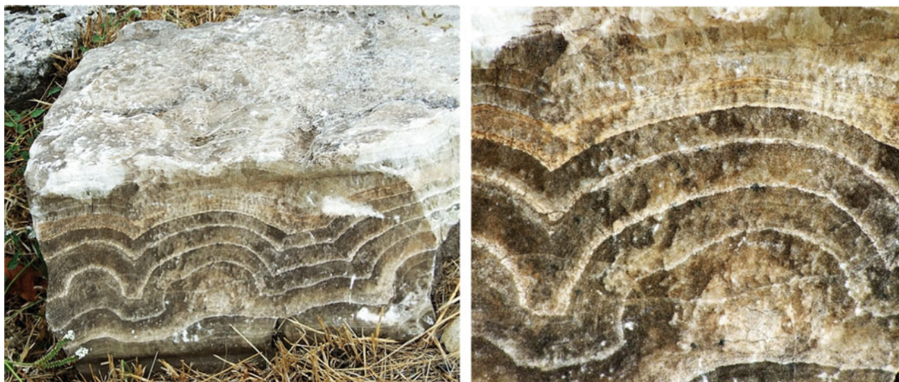
Fig. 10.19 Pamukkale travertine – a sample of ‘Hierapolis Stone’, a dense banded fissure travertine that was used as building material (sample on left c. 50 cm wide), also known as Phrygian Marble from Turkey
